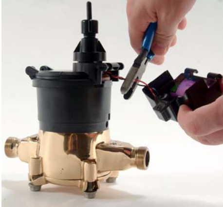
Figure 12 Cutting the Battery Wires
