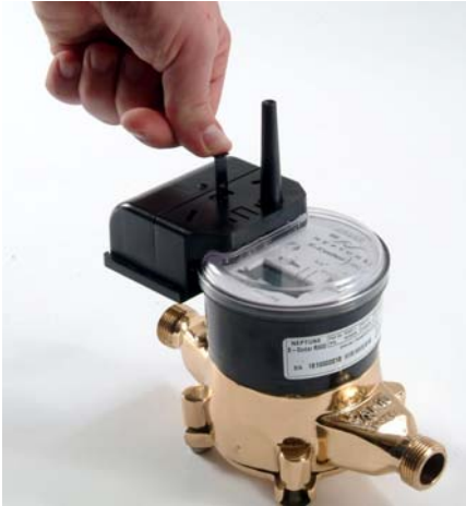
Figure 9 Pushing in New Tamper Nail
