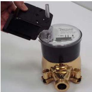
Figure 2 Sliding Battery over Antenna
