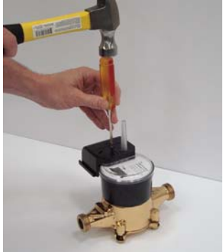
Figure 1 Screwdriver in Tamper Nail
