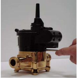
Figure 4 Screwdriver in Seal Pin
