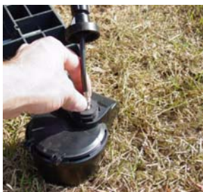
Figure 10 Connecting the Coaxial Cable
